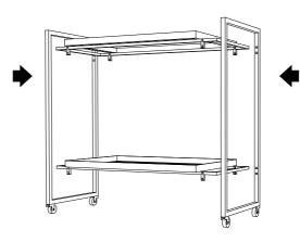
1. Place vertical frames in between the horizontal ones that all holes align.
