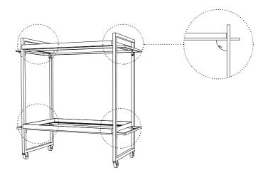
4. Aline the frame to create a right angle, than tighten all screws.
