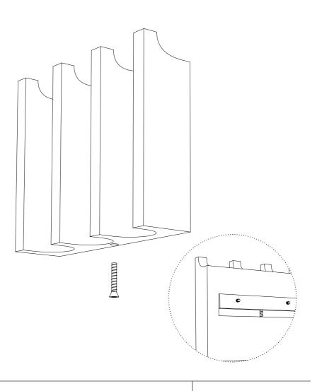
Scew the included screw with help of the Hex Key into the hole of the bottom of the Column Coat Rack. Tight the screw till it hits the wall bracket. It will help to hold the column coat rack safe to your wall.
