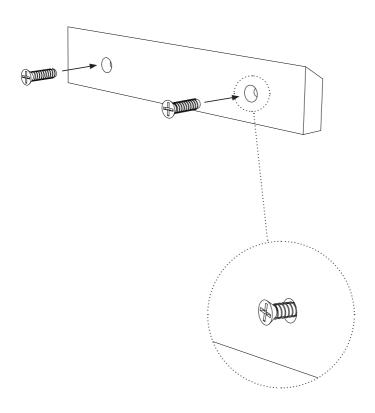
Screw the wooden bracket to the wall with 2 screws.
